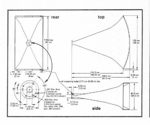
Electro-Voice® a gultan company Model HR4020A 40° x 20° **High Frequency** Horn
